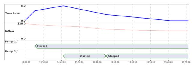
Remember that Stream B's objective is to control the Level to a set value, not to control the Flow leaving the Tank.
